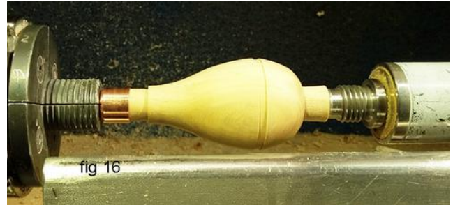
Fig. 16: Install the ferrule half way on, apply CA glue to all of the exposed wood that the ferrule will cover. Loosen the chuck grip and quickly press fit the ferrule the rest of the way on using the live centre / tailstock. Use epoxy if ferrule has a loose fit.
