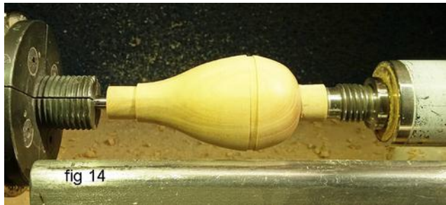
Fig. 14: Turn close to final shape – leave a bit to finish off later. Turn the tenon for the ferrule slightly over-sized
