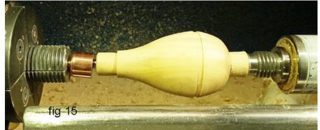
Fig. 15: Remount the work-piece with the ferrule added. Size the end of the handle so that the ferrule will need to be forced on. If it's a loose fit, use epoxy later to hold the ferrule in place.
