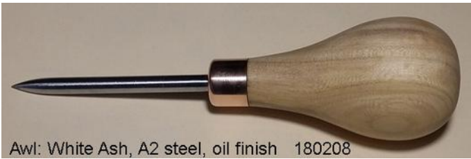
Fig. 19: Apply finish, allow to cure and you are done. Photo shows the finished awl with an Ash handle and a penetrating oil finish.
