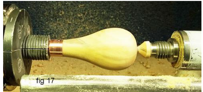
Fig. 17: Re-tighten the chuck. Turn the handle to final shape. Leave a small tenon on the end to keep the work-piece steady. Sand the handle. Sanding to 330 or 400 grit is more than enough.
