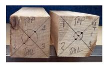
NOTE: the headstock markings are in a clockwise direction and the tailstock markings are in a counterclockwise direction.
