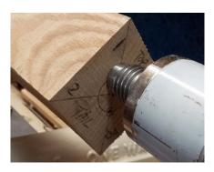
Bring up the tool rest even with the lathe ways, up to the blank – just make sure that the blank clears the tool rest as it will be swinging off centre.
