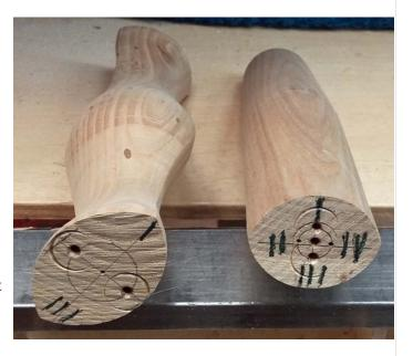
2.16 Now make a couple more, with different axis spacing and adding different shapes to become comfortable with this style of turning.
