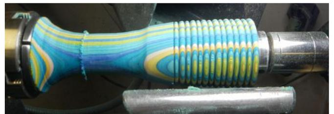
This photo shows orientation to turn the 'bottom' and most of the outside shape. After turning the bottom, you can apply the finish to that part of the body.
