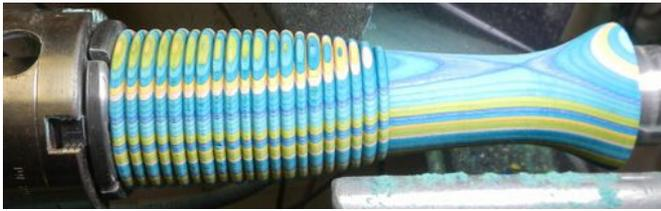
Turn the body around to final turn the 'top'. For safety and accuracy, use the tailstock with a cone or shop made accessory to hold the open end.
