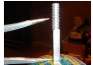
23. With the rod in the **{vise}** (protect rod from vise jaws), use a **{hammer}** to mushroom the four sides of the rod (at the non threaded end). The burrs must be large enough to keep the rod reliably in the mechanism. Be careful not to bend the rod.
