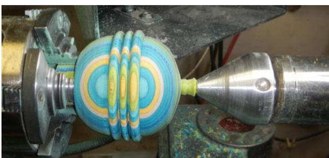
18. Sand the completed top, on the lathe, to 400 grit.
