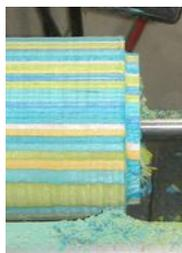
3. Part the cylinder stock into two pieces, a top and a body, according to your design. **{parting tool}** See photo in step 1. above for the proportions of the design in this example.
