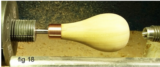
Fig. 18: Pull the live centre back and finish turning the end of the handle. Sand the end. If you wish to have a polished ferrule, pull the Awl back from the chuck and sand / polish.
