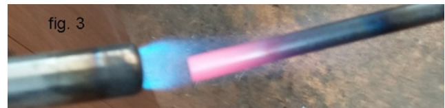
Fig. 3: Heat 1/2" (13mm) of rod end to cherry red, hold for 15 seconds, then quench immediately - moving the rod around - in cold water for a minimum of 30 seconds.
