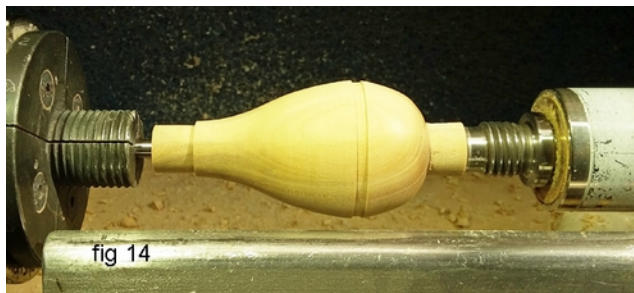
Fig. 14: Turn close to final shape – leave a bit to finish off later. Turn the tenon for the ferrule slightly over-sized
